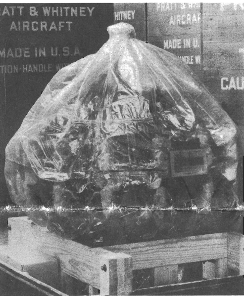
RAINCOAT FOR AN AIRCRAFT engine! This is how the Pratt and Whitney power plant, used in the F3A fighter which Brewster is building, looks when unpacked at Long Island. It is sealed in an airtight, Pliofilm envelope, which keeps out moisture. Inside the envelope, each cylinder has attached to it a dehydrating bag, while special cylinder plugs contain moisture-absorbing crystals.
