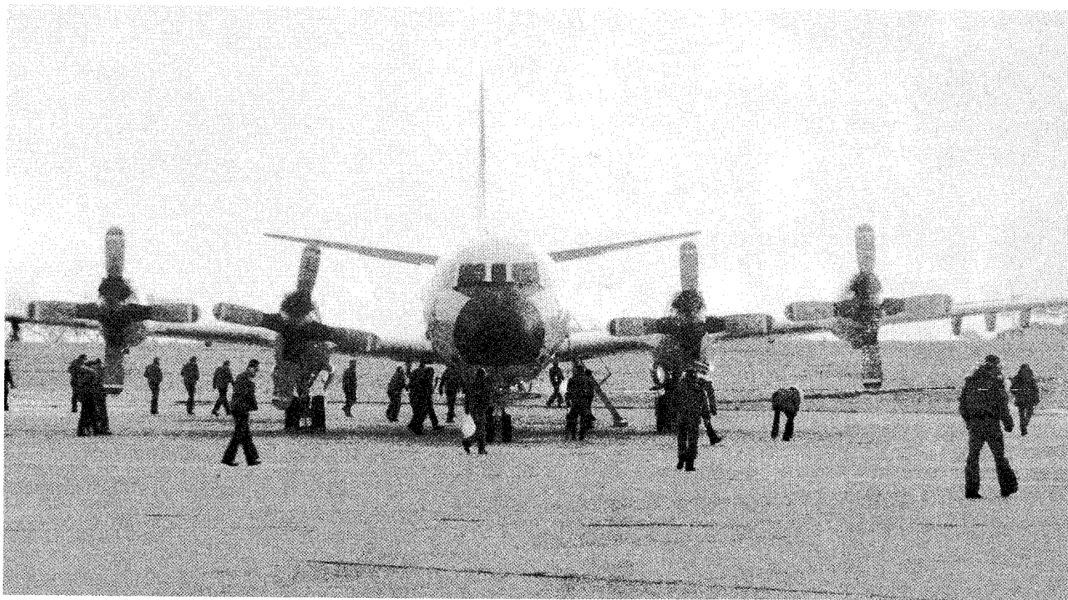
Under and around parked aircraft, the FOD crew scours ever inch of the area.
