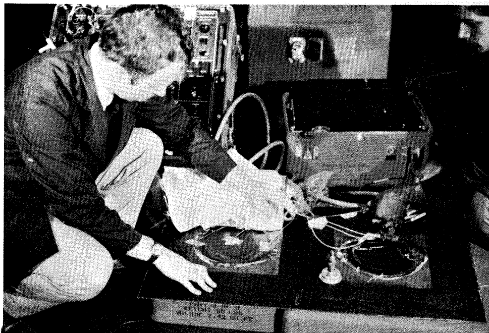
Tom Donnellan (left) and Roland Cochran (right), Code 6063, removing vacuum bag from composite repair.
