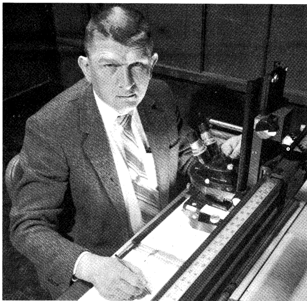
Harry Koper sits at light table to read resolution of camera lens on test film.
