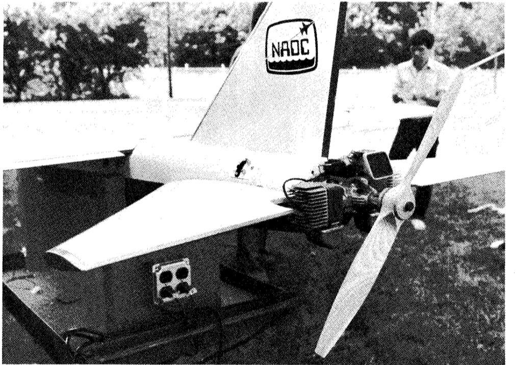
RPV's 4.5 HP, 2-cylinder model A/C engine.
