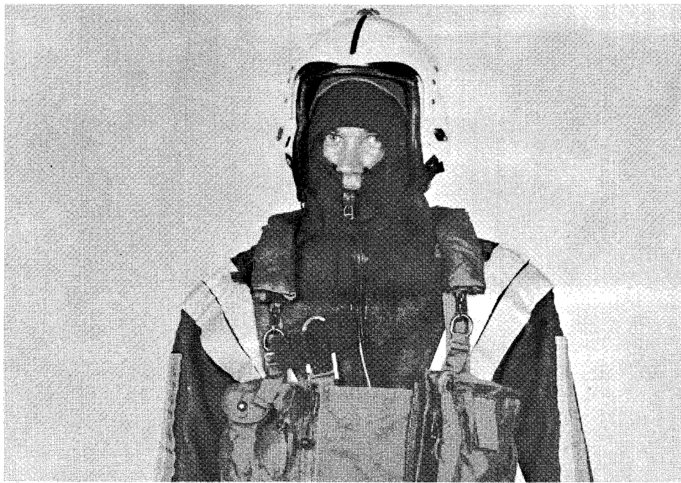
The CWU-60/P quick-donning anti-exposure suit, soon to be introduced to the Fleet, is an example of the Life Support Equipment Division's work supported by the FAILSAFE program.
